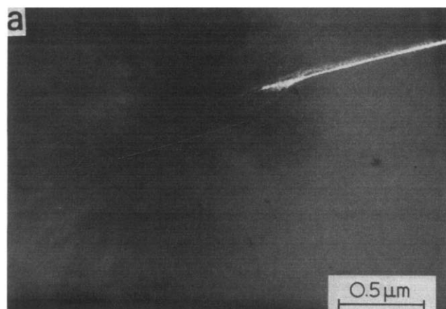
Figure 21 Electron micrograph of a Type IV interaction showing the craze tip inside the spherulite
